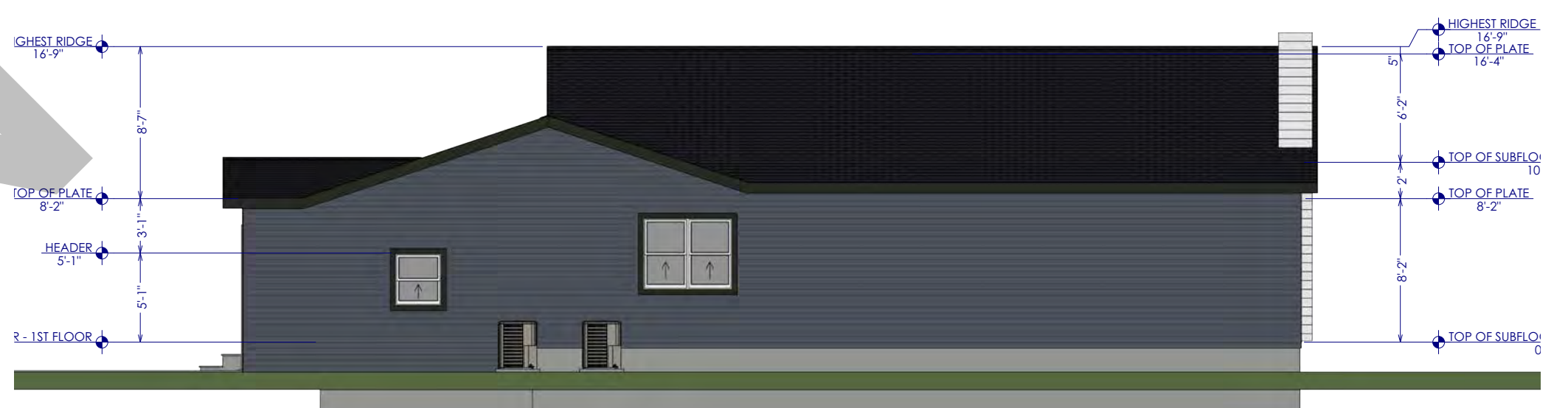
E22 EAST ELEVATION 3/16 in = 1 ft
